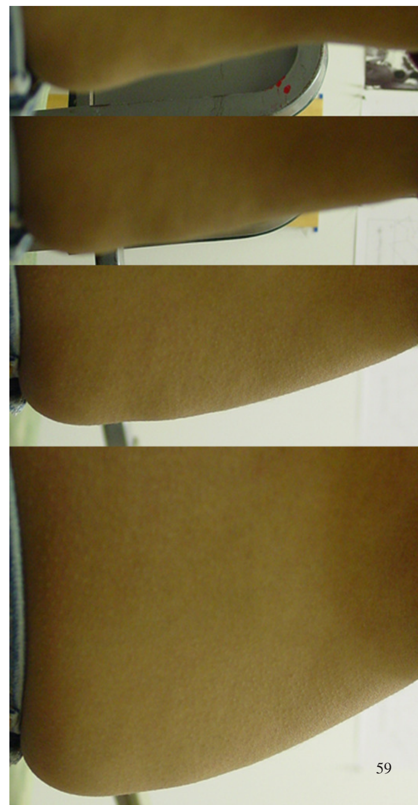
27 Study model of a sagging roof in the community space: the roof is made of lycra and collects rain water. The membrane sags as the water content increases and has a degree of porosity by which, after it gets saturated, it drips and collects in the water pool below. This forms the central feature of the community space and a sign of sustainable architecture.
